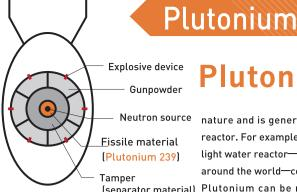
Length: 3.25 m; Diameter: 1.52 m; Weight: 4.5 tons Nicknamed "Fat Man"
