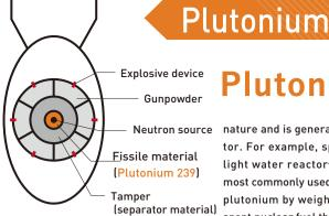
Length: 3.25 m; Diameter: 1.52 m; Weight: 4.5 tons Nicknamed "Fat Man"
